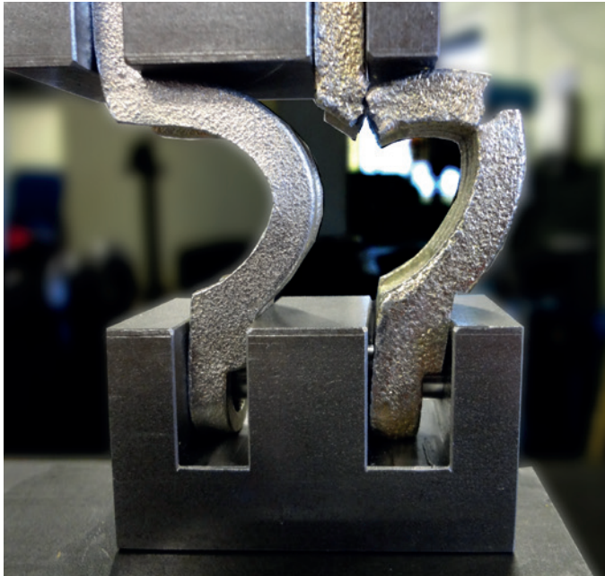
Fracture test - left: LUDKE hose clamp (no crack/ fracture), right: hose clamp from the Far East (complete fracture)
