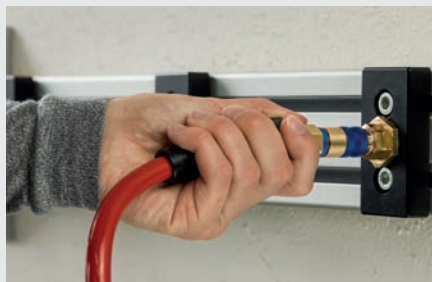
One-hand operation: To connect, push the plug into the coupling. (The colours of the aluminium sleeve of the coupling and the aluminium ring of the plug as well as the plug-coding have to be identical.)
