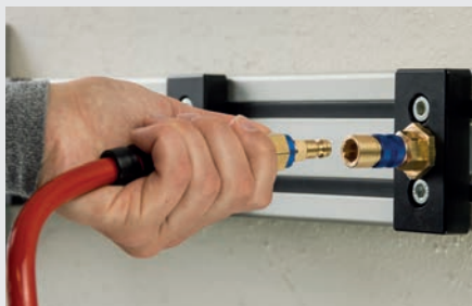
One-hand operation: To connect, push the plug into the coupling. (The colours of the aluminium sleeve of the coupling and the aluminium ring of the plug as well as the plug-coding have to be identical.)
