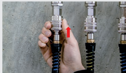
Disconnection - first step: Automatic venting
