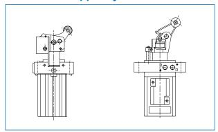
The built-in shock absorber softly catches and stops the work carrier. The strength of absorber can be easily adjusted, which makes the cylinder work in the best condition, conforming to the speed of the conveyor line and the weight of the work carrier.
