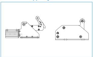
orizontal stopper cylinder of lower height for conveying the heavy work carriers. Suitable as a stopper cylinder for accumulating line, ageing line, and mulit-stage conveyor line. Softly stops the work carriers of heavy weight and high speed.
