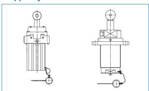
The top rollers with the built-in spring return in touch with the bottom of the work carrier. Automatically returns up to the original position as the work carrier pass by, and immediately works as a stopper for the next work carrier. Therefore the timing carriers does not need to be taken.
