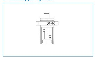
Rod and cylinder are designed for toughness against the large side load. Also suitable for the relatively slowmoving conveyor line with the heavy work carriers.
