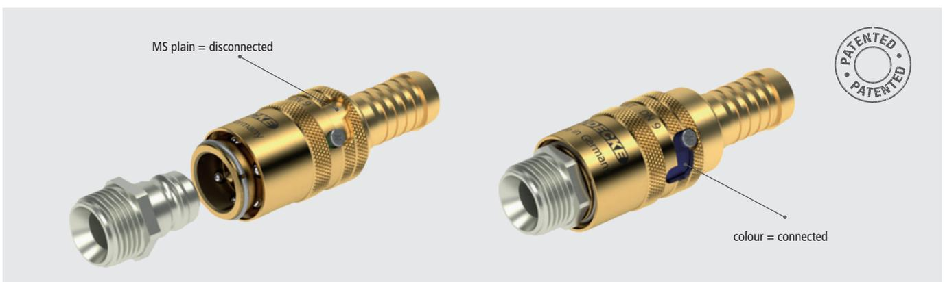
The disconnecting process can be performed blindly due to the forced guidance of the locking sleeve. However, this requires a deliberate manual unlocking effort. An accidental or unintentional disconnection is almost impossible.
